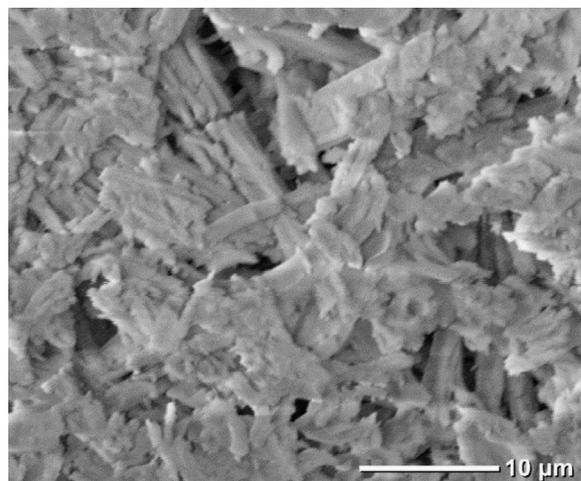
Fig. 1. SEM image of a gypsum fragment.
