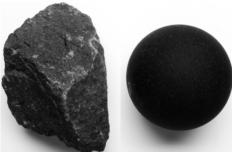
Fig. 2. Our typical irregularly-shaped and spherical basalt targets. The natural, irregularly-shaped targets are hand specimens collected in the field from the sample site. The spherical targets we prepared from larger fragments of the same basalt; the darker color is due to infusion of lubricating oil used during the milling process to obtain the spherical shape. The targets shown here were not shot during this experiment run; they remain for future impact experiments.
