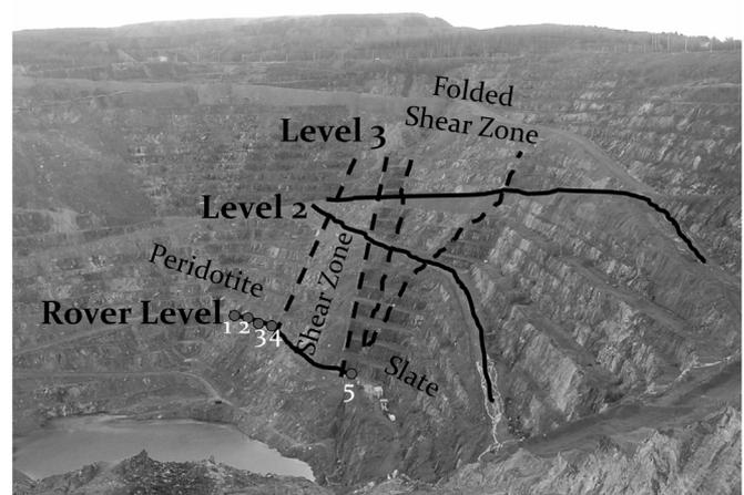
**Fig. 1.** Interpreted photo of the open-pit Jeffrey Mine showing geological contacts (dashed lines), the locations of EMIS surveys (solid lines), and laser imaging sites (numbered dots).
