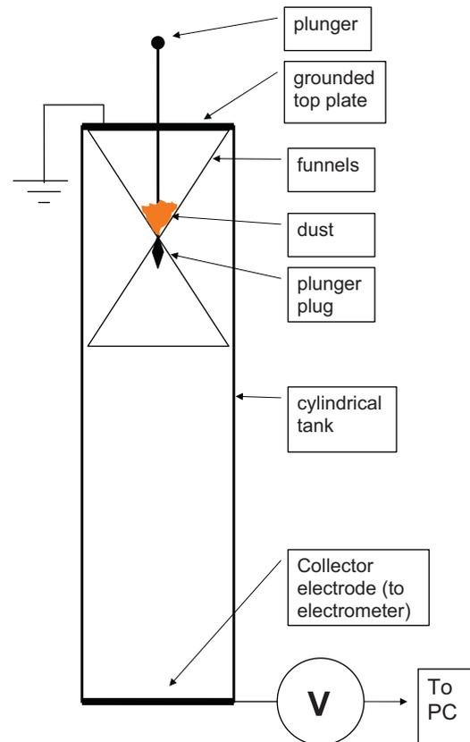
**Fig. 1.** Apparatus showing the Martian analogue material loaded before a drop (dust drops are activated by pushing down the plunger). The cylindrical tank is mounted on a support frame which permits the tank to be rotated to re-load the Martian analogue material. The carbon dioxide gas supply line and vacuum pump (not shown) are disconnected before each dust drop and rotation, and the tank sealed with a valve.
