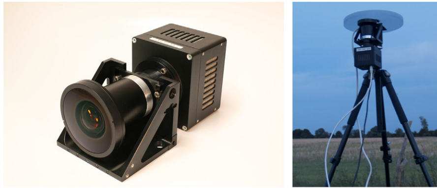
Fig. 1. SPOSH breadboard camera head (left). SPOSH camera mounted on a tripod at dusk, equipped with a rotating shutter (right).
