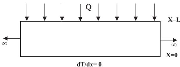
Fig. 1. One-dimensional step heating of heat conduction problem.
