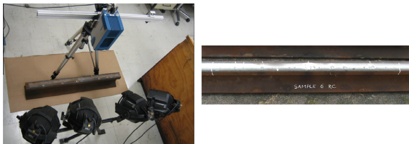
Fig. 2. Experimental setup of the lock-in thermographic equipment and specimen.
