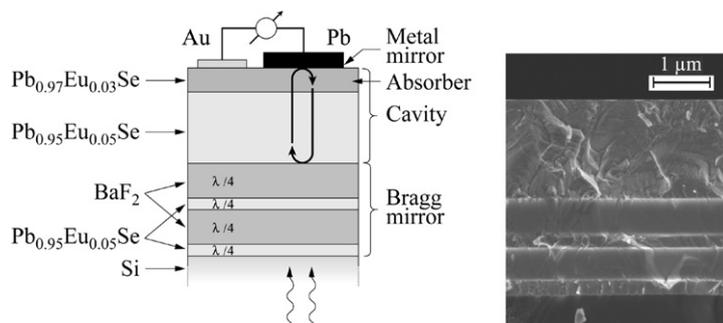
Fig. 2. Schematic cross section of a lead-chalcogenide RCED and corresponding scanning electron microscopic image.
