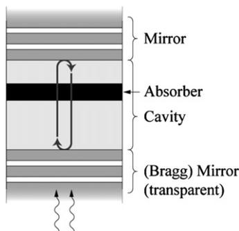
Fig. 1. Principle of a RCED.
