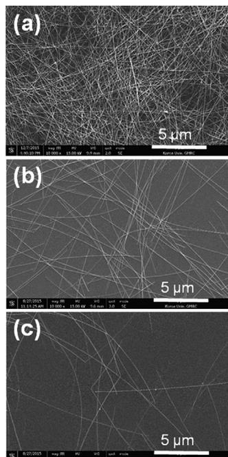
**Fig. 1.** SEM images of Ag NWs on ITO films (10 nm thick) coated at a speed of (a) 500, (b) 1000, and (c) 3000 rpm. Schematic of 3-D LEDs fabricated (d) with ITO-only and (e) ITO/Ag NW electrodes.
