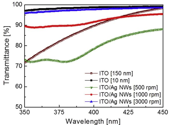
**Fig. 2.** The optical transmittance of 150 nm-thick ITO, 10 nm-thick ITO and ITO (10 nm)/Ag NWs films deposited at different coating speeds.
