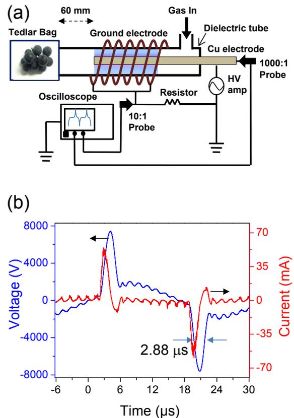
Fig. 1. (a) Schematic diagram of experimental set-up for atmospheric-pressure dielectric barrier discharge system and (b) waveforms of applied voltage and current at input voltage of 120 V and air gas flow rate of 15 L/min.
