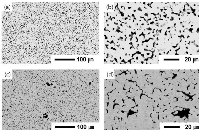
Fig. 1. Scanning electron microscopy (SEM) images of the sintered tungsten (W) billet: (a) sample created using metal injection molding (MIM) (500 $\times$ ), (b) an enlarged MIM sample (2000 $\times$ ), (c) sample created using die pressing (500 $\times$ ), and (d) enlarged die-pressed sample (2000 $\times$ ).
