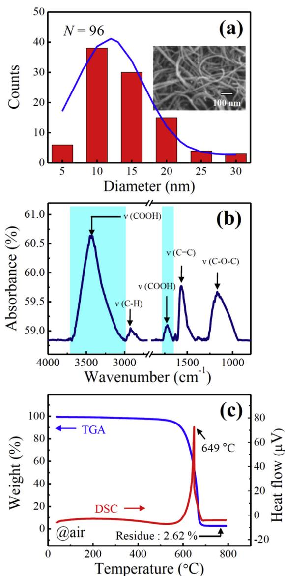
**Fig. 1.** (a) A graph of the MWCNTs diameter distribution and inset image of FESEM images showing functionalized MWCNTs, (b) FTIR absorbance spectra, and (c) TGA and DSC spectra of functionalized MWCNTs.
