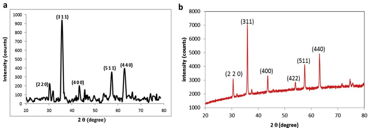
Fig. 2. XRD measurement for cobalt ferrite (a) and cobalt nickel ferrite (b) showing the formation phase pure product with particle size 20 nm (a) and 25 nm (b).
