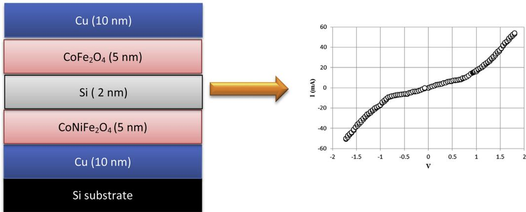
Fig. 1. Schematic representation of magnetic junction.  $I$ - $V$  plot of this junction shows non-linear behavior.
