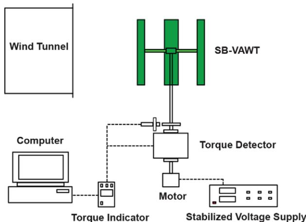
Fig. 2. Schematic diagram of experimental system.
