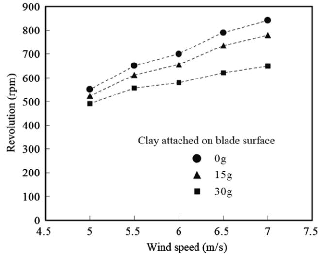
Fig. 3. Steady revolution at different wind speeds.
