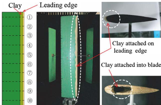
Fig. 1. Position of clay attached on or in blade.
