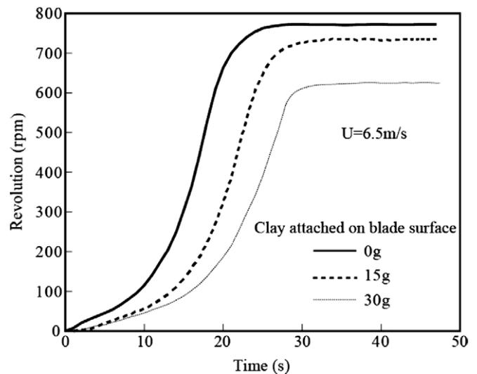
Fig. 4. Revolution changes at wind speed U = 6.5 m/s.
