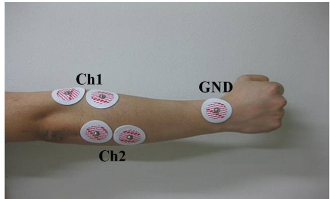
Fig. 2. The two-channel-electrodes positions of the right forearm.
