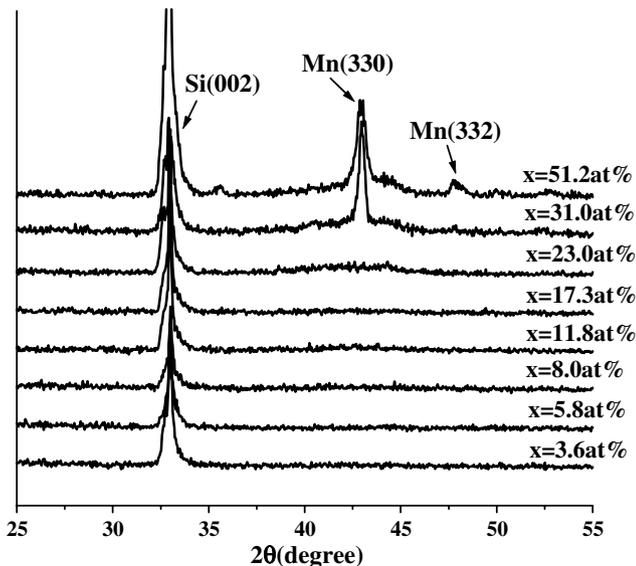
Fig. 1. X-ray diffraction patterns of  $\text{Ge}_{1-x}\text{Mn}_x$  films.
