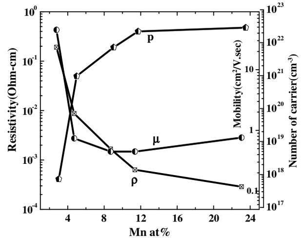
Fig. 3. Hall data of  $\text{Ge}_{1-x}\text{Mn}_x$  thin films measured at room temperature.
