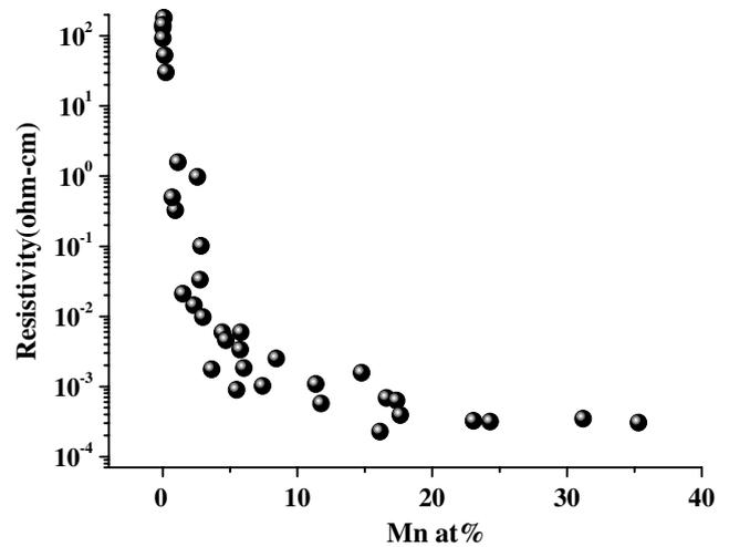
Fig. 2. Sheet resistivities of  $\text{Ge}_{1-x}\text{Mn}_x$  semiconductor thin films measured at room temperature using four-point probe.
