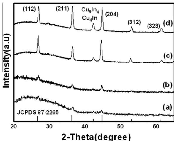
Fig. 1. X-ray diffraction patterns of the CuInSe<sub>2</sub> thin films annealed at 400 °C for 1 h: (a) the as-deposited, (b) 0.005 M of InCl<sub>3</sub>, (c) 0.010 M of InCl<sub>3</sub> and (d) 0.025 M of InCl<sub>3</sub> in the precursor solution of In source.
