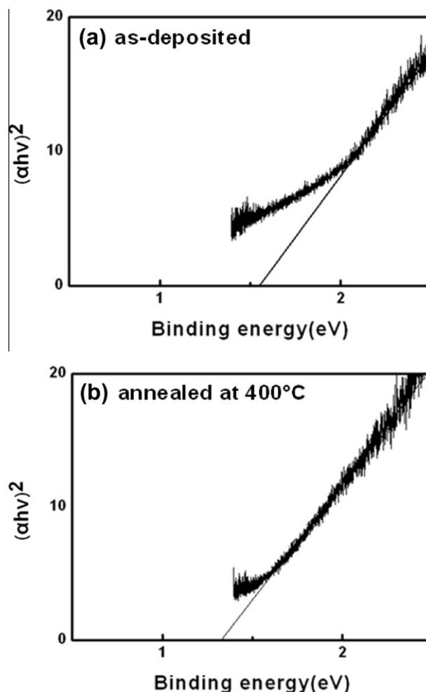
Fig. 2. UV–vis absorption spectra of the CuInSe<sub>2</sub> film deposited with the precursor solution containing 0.025 M of InCl<sub>3</sub> and its estimated optical band gap: (a) the as-deposited and (b) the annealed at 400 °C.
