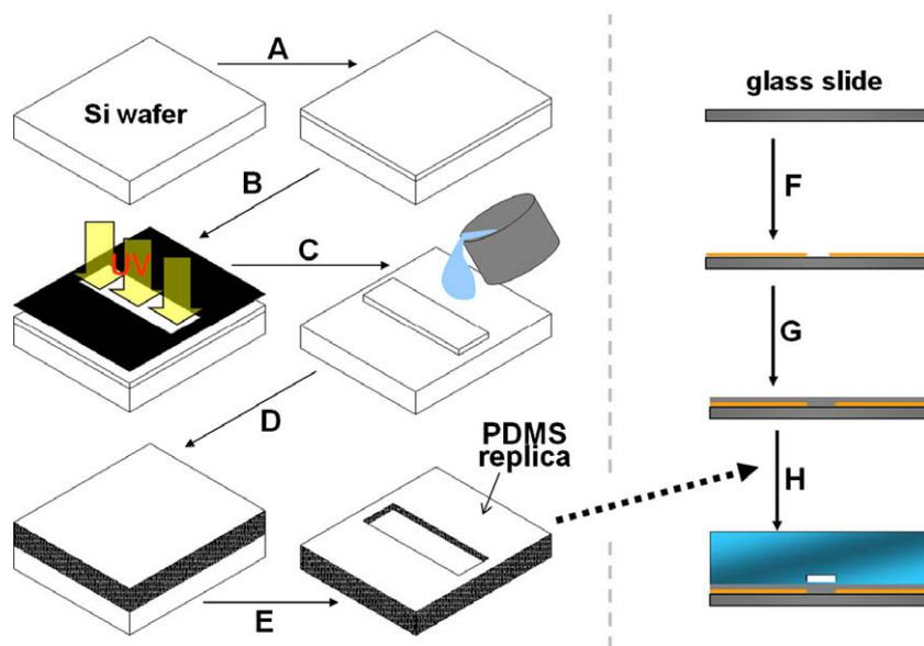
**Fig. 1.** Fabrication process of the PDMS microfluidic device using photolithography and replica molding: (A) negative PR (SU-8) spin-coating; (B) UV exposure with contact mask; (C) developing; (D) applying PDMS on master PR pattern and curing PDMS at 70 °C; (E) detaching PDMS from master pattern; (F) electrode patterning on a glass slide; (G) TEOS-sol spin-coating; (H) alignment and bonding between PDMS mold and glass substrate.
