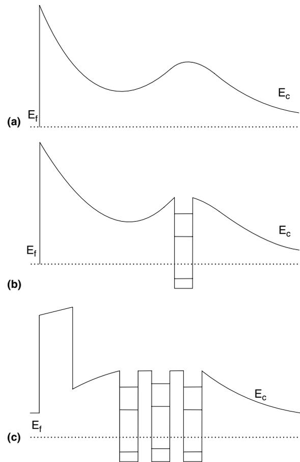
Fig. 1. Schematic diagram of the conduction band, for (a) the reference Schottky diode, (b) the Schottky diode with a QD layer, and (c) the n-i-n diode with three QD layers and an AlGaAs current blocking layer.
