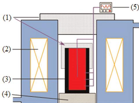
Fig. 1. Schematic diagram of the experimental apparatus: (1) asbestos, (2) TMF coils, (3) graphite crucible, (4) firebrick, and (5) temperature measurement system.
