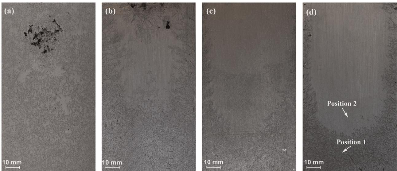
Fig. 2. Morphologies of Al–30Si ingot solidified under TMF with different magnetic flux densities: (a) 0 mT, (b) 10 mT, (c) 25 mT, and (d) 50 mT.
