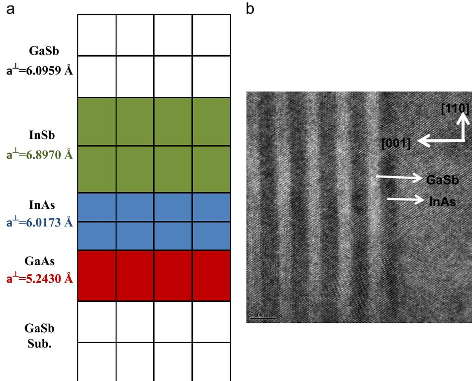
Fig. 1. (a) The schematic drawing showing the pseudomorphic growth of a type II SL structure with the vertical lattice constant denoted for GaAs, InAs, InSb and GaSb materials. (b) The cross-sectional TEM image of sample e.
