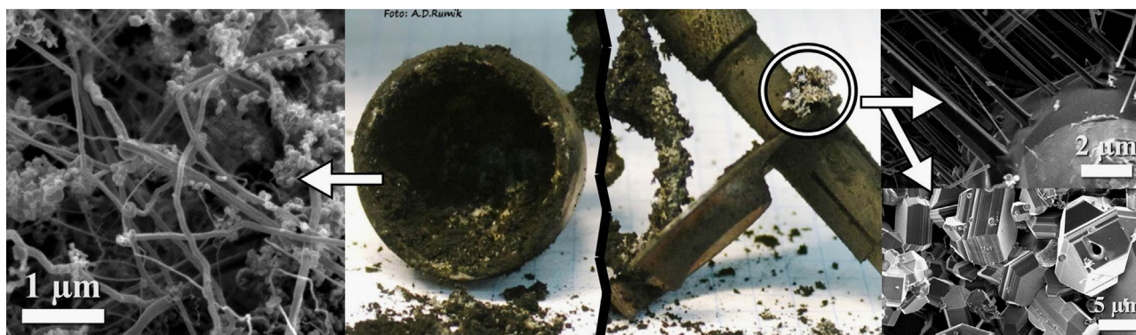
Fig. 1. The morphology of the products; Left—typical fibers in the spongy form of the product, right—dense fragments of different morphology at the nano level.
