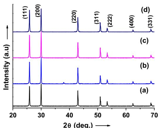
Fig. 1. XRD spectra of the products in en with reaction time of 6 h and reaction temperature of 180 °C assisted by L-cysteine of different concentration, (a) 0 mmol; (b) 0.01 mmol; (c) 0.02 mmol; (d) 0.05 mmol.
