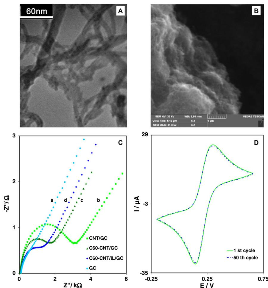
Fig. 1. (A) TEM image of  $C_{60}$ -CNT, (B) SEM image of  $C_{60}$ -CNT/IL nanocomposite, (C) Nyquist plots of bare GC electrode (a), CNT/GC (b),  $C_{60}$ -CNT/GC (c),  $C_{60}$ -CNT/IL/GC, (D) 1st cycle and 50th cycle of  $C_{60}$ -CNT/IL/GC in 1 mM  $\text{Fe}(\text{CN})_3^{+/4-}$  containing 0.1 M KCl.
