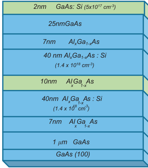
Fig. 1. Layers structure of sample M3. M2 does not have the capping layer (2 nm–GaAs:Si). M1 does not have two layers: 10 nm–AlGaAs and 2 nm–GaAs:Si. Aluminum concentration for all samples was x=0.36 .
