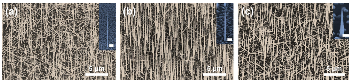
Fig. 1. SEM images of ternary \text{In}_x\text{Ga}_{1-x}\text{As} NWs grown at: (a) 440, (b) 470, and (c) 500 °C, respectively. Insets in the figure are the high magnification SEM image of the NWs with 500 nm of scale bar. The NWs are more tapered as the growth temperature increases indicating that more sidewall growth is activated.
