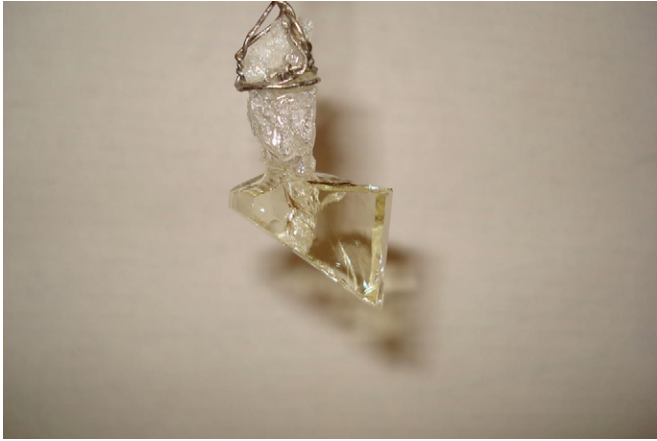
Fig. 1. LCBO:Pr 3+ single crystal grown from melt containing 4 at% of Pr 3+ ions in the melt.
