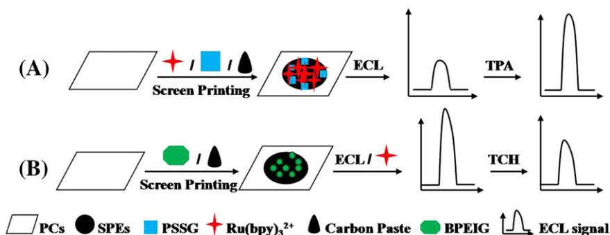
Fig. 1. Schematic illustration of preparation and application for solid-state (A)  $\text{Ru}(\text{bpy})_3^{2+}$  and (B) coreactant ECL sensors.
