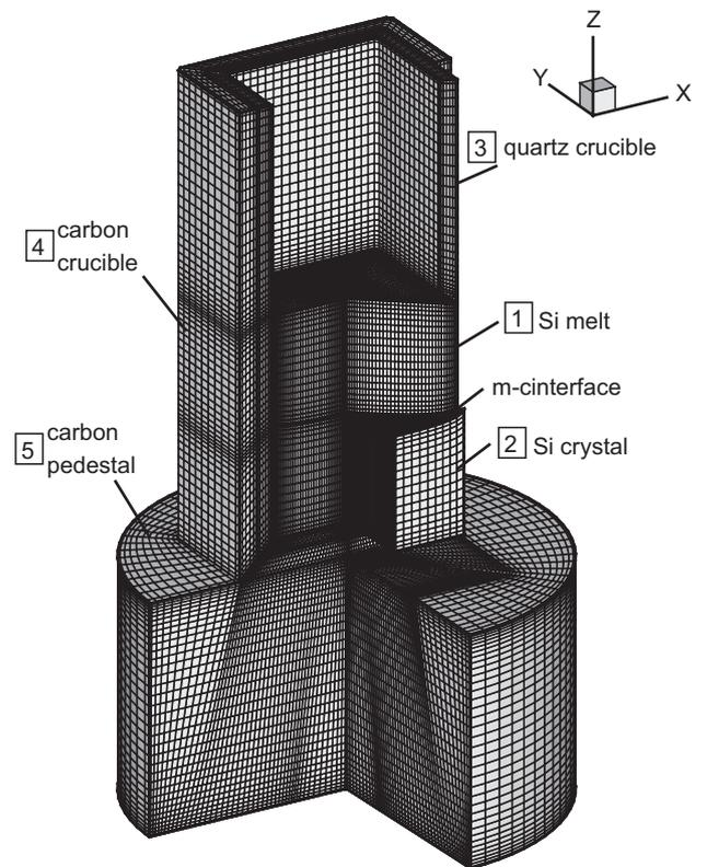
Fig. 2. Three-dimensional computation grid used for the 3D global model.
