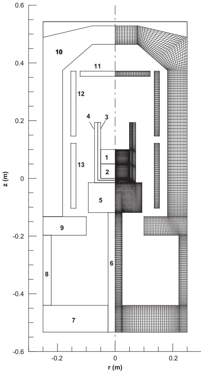
Fig. 1. Configuration and computation grid of a unidirectional solidification furnace with cylindrical crucibles.
