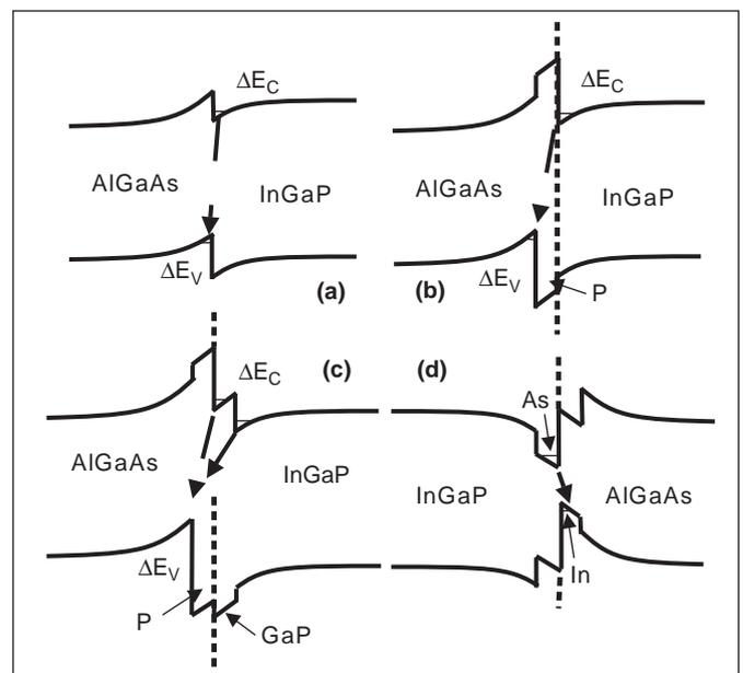
Fig. 2. Schematic band structures with various InGaP-on-AlGaAs interfaces. (a)—ideal, (b)—with AlGaP interlayer, (c)—with AlGaP and GaP interlayers) and AlGaAs-on-InGaP one (d).
