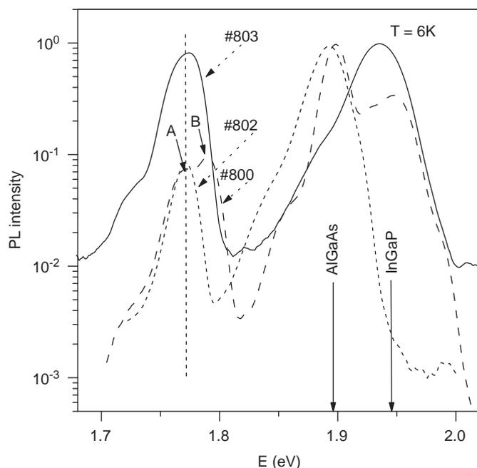
Fig. 1. PL spectra of the structures without a GaP interlayer (#803) and with GaP interlayers (#800, #802).
