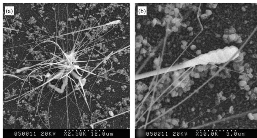
Fig. 2. (a) The image of nanowires cluster obtained at  $950^\circ\text{C}$ , and (b) the amplified image of a part of cluster.
