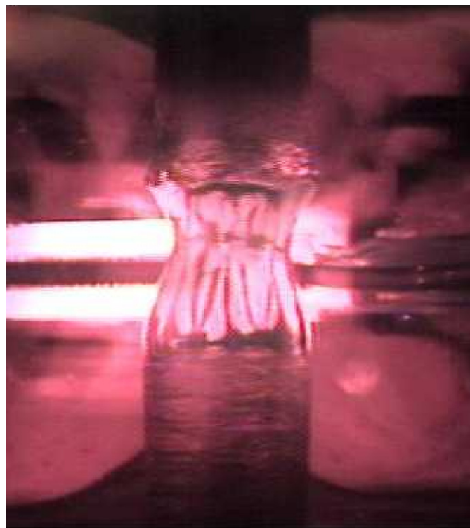
Fig. 2. The shape of the zone in the growth of \text{La}_{0.04}\text{Sr}_{0.96}\text{Cu}_2(\text{BO}_3)_2 crystal from premelted rod with the speed of 0.25 mm/h in \text{O}_2 .
