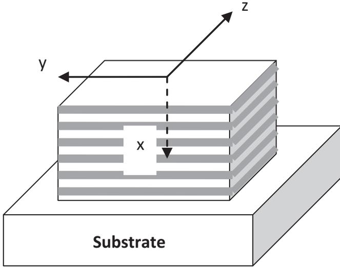
**Fig. 1.** Geometry of anisotropic periodic structure with layers perpendicular to the x-axis.
