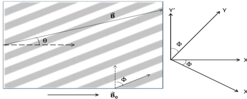
**Fig. 2.** Cross-section of the multilayer composite in the  $x'y'$ -plane with layers rotated on angle  $\varphi$  around the z-axis;  $\theta$  is the bending angle of the magnetic flux density.
