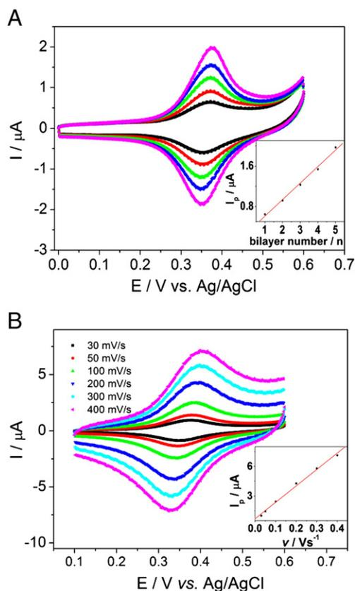
**Fig. 1.** (A) Current responses of the Au/MPA/(Fc-PAH/SWNT)<sub>n</sub> electrode in 0.9% NaCl supporting electrolyte. n = 1, 2, 3, 4, 5 from inner to outer. Scan rate: 50 mV/s. Inset shows linear dependence of peak current on increasing number of bilayer (Fc-PAH/SWNT). (B) Current responses of the Au/MPA/(Fc-PAH/SWNT)<sub>5</sub>/PAH electrode with different scan rates in 0.9% NaCl supporting electrolyte. Inset shows linear dependence of the peak current on scan rate.
