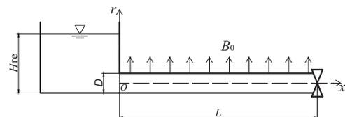
Fig. 1. The physical model of MHD fluid hammer.
