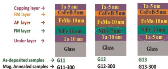
Fig. 1. The schematics of the deposited samples.
