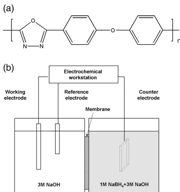
Fig. 1. (a) Chemical structure of POD-DPE; (b)  $\text{BH}_4^-$  permeability measurement device comprising a diffusion cell and a three-electrode system.
