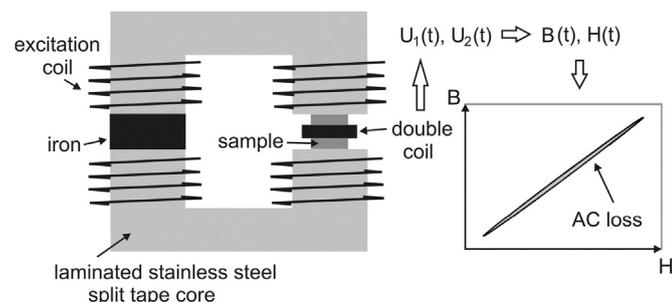
Fig. 1. Schematic of magnet yoke for AC loss measurements.
