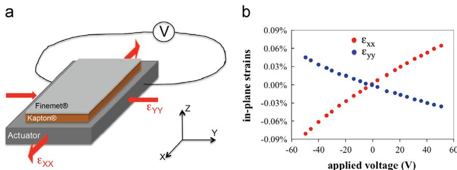
**Fig. 2.** (a) Sketch of the artificial FeCuNbSiB/piezoelectric heterostructure. (b) Quantitative characterization of the voltage dependence of the induced-strain at the surface of the film performed using a digital image correlation technique.
