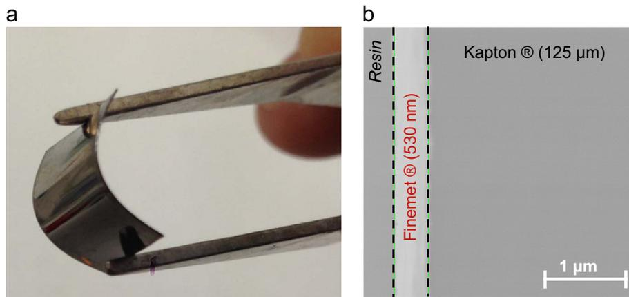
**Fig. 1.** (a) Image of the flexible Finemet/Kapton<sup>®</sup> system. (b) Cross-section of the Finemet/Kapton<sup>®</sup> system obtained by a scanning electron microscope (SEM). A Finemet film thickness of about 530 nm is estimated.
