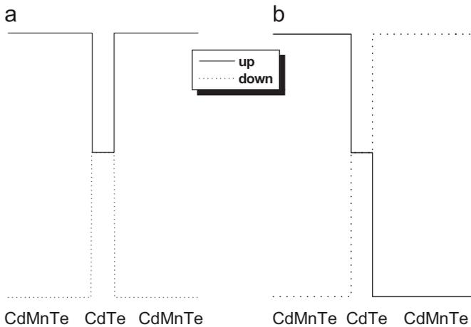
Fig. 1. Potential profiles for spin-up and spin-down in the ferromagnetic (F) and anti-ferromagnetic (AF) configurations, respectively, for a tri layers quantum well.
