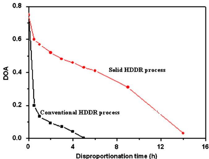
Fig. 1. Effects of disproportionation time on DOA of conventional and solid HDDR  $\text{Pr}_{13}\text{Fe}_{80}\text{B}_7$ -bonded magnet.
