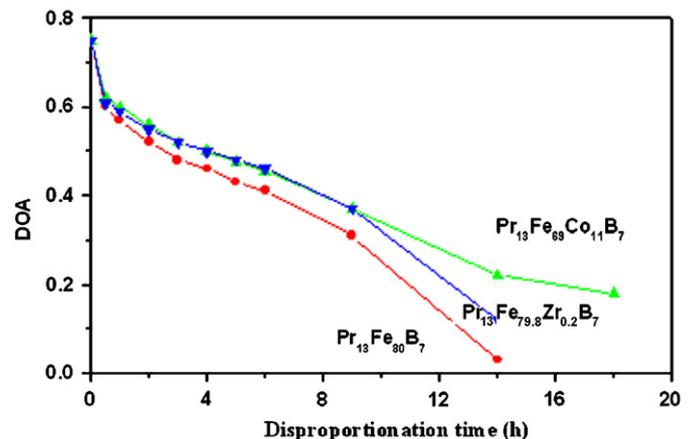
Fig. 2. Effects of disproportionation time on DOA of solid HDDR  $\text{Pr}_{13}\text{Fe}_{80}\text{B}_7$ ,  $\text{Pr}_{13}\text{Fe}_{69}\text{Co}_{11}\text{B}_7$  and  $\text{Pr}_{13}\text{Fe}_{79.8}\text{Zr}_{0.2}\text{B}_7$  bonded magnet.
