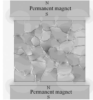
Fig. 2. Magnetic-flux density distribution in the ferromagnetic particles.
