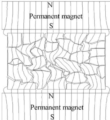
Fig. 1. Distribution of magnetic-flux lines in the ferromagnetic particles.
