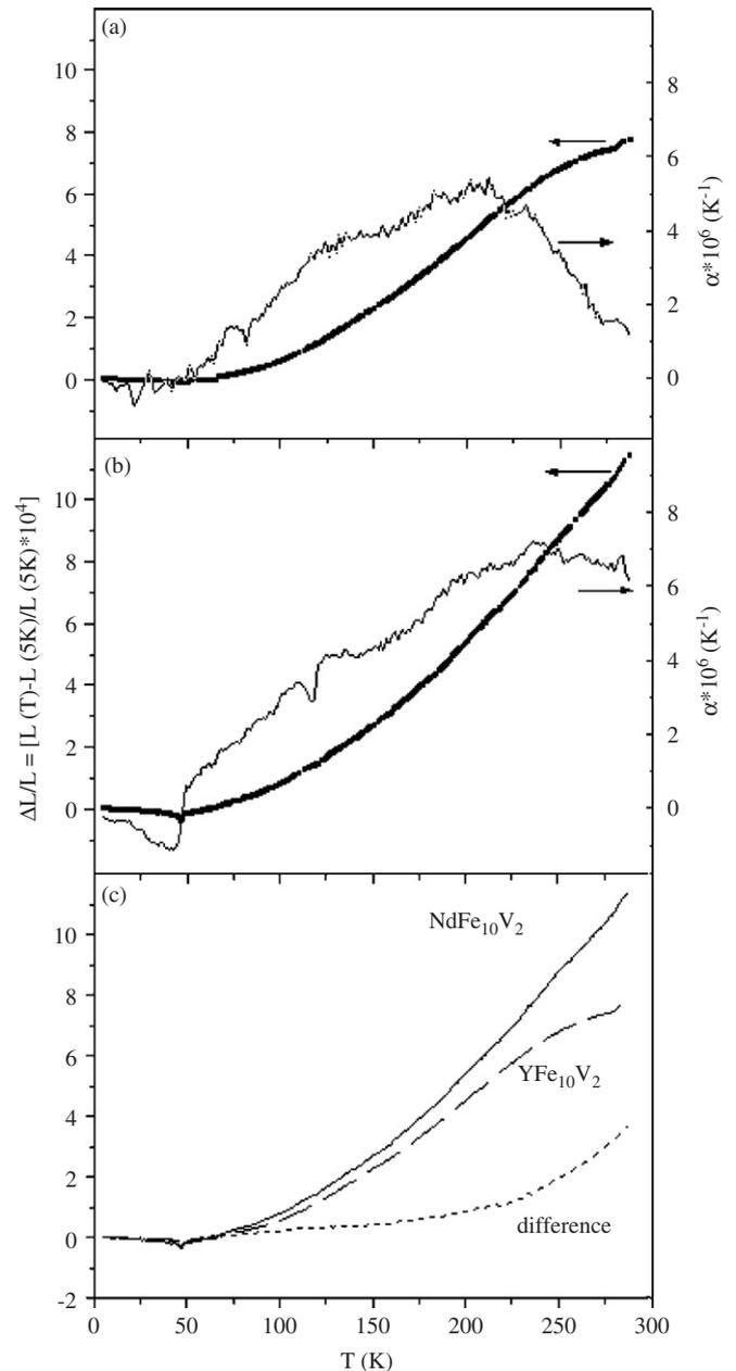
Fig. 1. Thermal expansion of (a)  $\text{YFe}_{10}\text{V}_2$ , and (b)  $\text{NdFe}_{10}\text{V}_2$  and corresponding coefficients  $\alpha \equiv (d/dT)(\Delta L/L)$ . (c) Difference of the thermal expansion between the two studied compounds.
