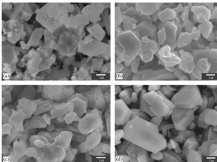
Fig. 1. SEM micrographs of Sr-ferrite powders synthesized at  $800^\circ\text{C}$  for different reaction times: (a) 10 min; (b) 1 h; (c) 2 h; and (d) 6 h.
