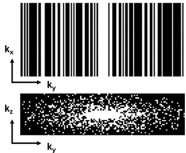
Fig. 1. The associated variable density undersampling scheme in k x -k y plane (top) and the cross-section of randomly undersampling in k z -k y plane (bottom) for CS-combined MRI.
