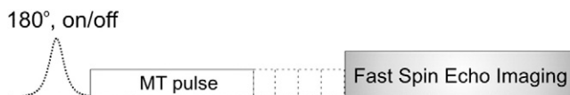
Fig. 1. Pulse sequence for the described MT protocol. The frequency of the MT pulse is 6 kHz off-resonance, and the peak amplitude ( \gamma B_1/2\pi ) is 150 Hz for human studies. The dashed squares indicate incremental durations of the MT pulse, which is applied immediately prior to the excitation pulse of the imaging module. The MT measurement is performed twice, with and without an on-resonance inversion pulse prior to the off-resonance irradiation, with no time delay. The time between the inversion pulse and the excitation pulse of the imaging module is determined by the duration of the MT pulse, thus leading to inversion recovery that occurs entirely in presence of the off-resonance irradiation. In this study, the imaging module consisted of a fast SE readout with 90° excitation, while the MT pulse consisted of CW irradiation. However, other types of imaging readout are possible, as well as other pulsed approaches can be implemented instead of CW irradiation to achieve the off-resonance saturation.
