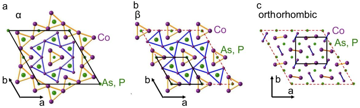
**Fig. 1.**  $\text{Co}_2\text{As}_{1-x}\text{P}_x$  crystal structure for (a) the hexagonal  $\alpha$  phase, (b) the hexagonal  $\beta$  phase, and (c) the orthorhombic phase. The unit cell is indicated by the black solid line, and the red dashed parallelograms are used as a comparison with the hexagonal  $\alpha$  phase. (For interpretation of the references to color in this figure caption, the reader is referred to the web version of this paper.)
