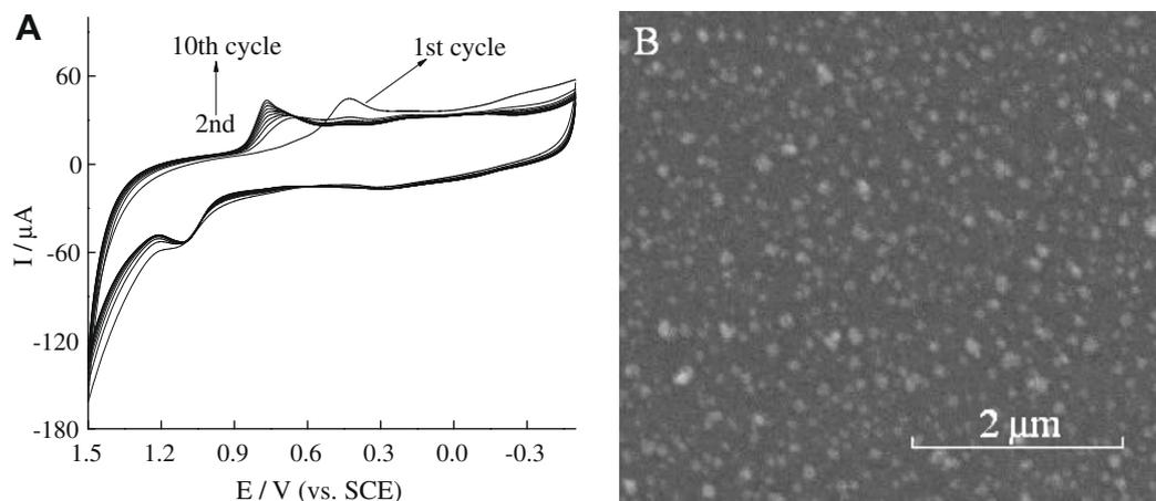
**Fig. 1.** A: Cyclic voltammograms recorded at IL-SWNT/GCE immersed in the 0.01 M  $\text{Na}_2\text{SO}_4$  containing 0.01 M  $\text{H}_2\text{SO}_4$  and 0.5 mM  $\text{HAuCl}_4$  solution at scan rate of 100 mV/s. B: SEM image of GNP-IL-SWNT with 10-cycle deposition.
