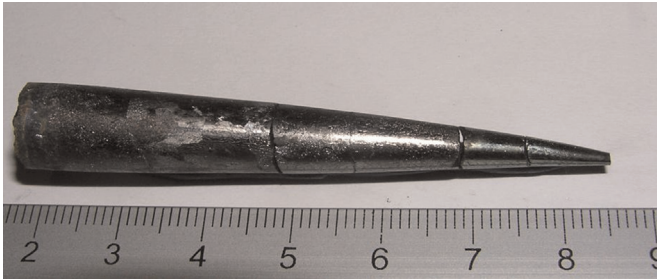
Fig. 1. Photo of as-grown boule containing \text{Cu}_2\text{ZnGeSe}_4 single crystal used in the present experimental studies.
