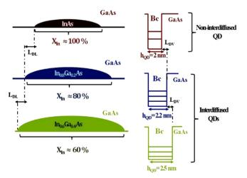
**Fig. 1.** Schematic model of a lens-shaped interdiffused InAs QD for different indium compositions.
